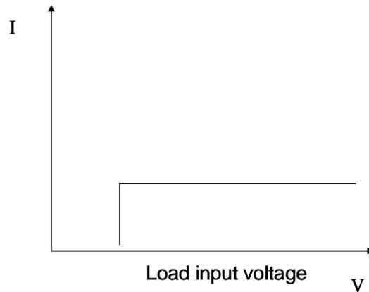
Diagram 4.4 Constant Current Shift Mode back into Constant Voltage Mode
